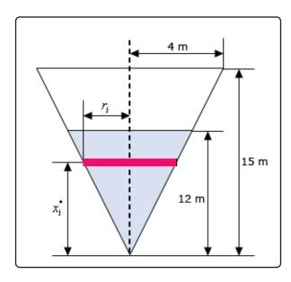
The red strip in the sketch represents the "cylinder" of water in the  $i^{th}$  subinterval. A quick application of similar triangles will allow us to relate  $r_i$  to  $x_i^*$  (which we'll need in a bit) as follows.
