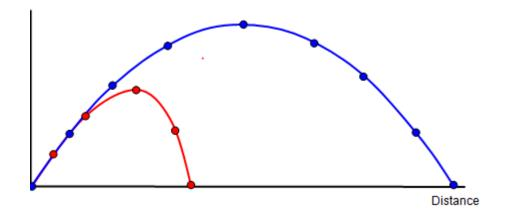
We will perform an experiment in which we will use the formula for the range of a projectile (in the presence of air resistance) to find out the damping coefficient (b) of air.
