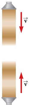
Figure 18.6 Two identical loudspeakers emit sound waves toward each other. When they overlap, identical waves traveling in opposite directions will combine to form standing waves.
