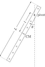
We define the total length of the bar as L and the distance from the pivot to the center of mass (CM) of the bar to be l as indicated in the diagram above. The position of the bar at any instant of time is given by the angle  $\theta$ . When allowed to swing the bar performs an approximation of simple harmonic motion, that is, the angle  $\theta$  varies in a cyclic fashion with time period T.
