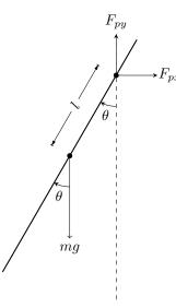
There are two forces acting on the bar. Its weight, which acts at the bar's center of mass/gravity, and a force of unknown magnitude and direction acting at the pivot,  $\vec{F_p}$ .
