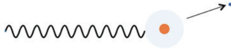
Fig. 5.4 Photoelectric effect. Note that the photon is absorbed by the atom, which expels an electron
