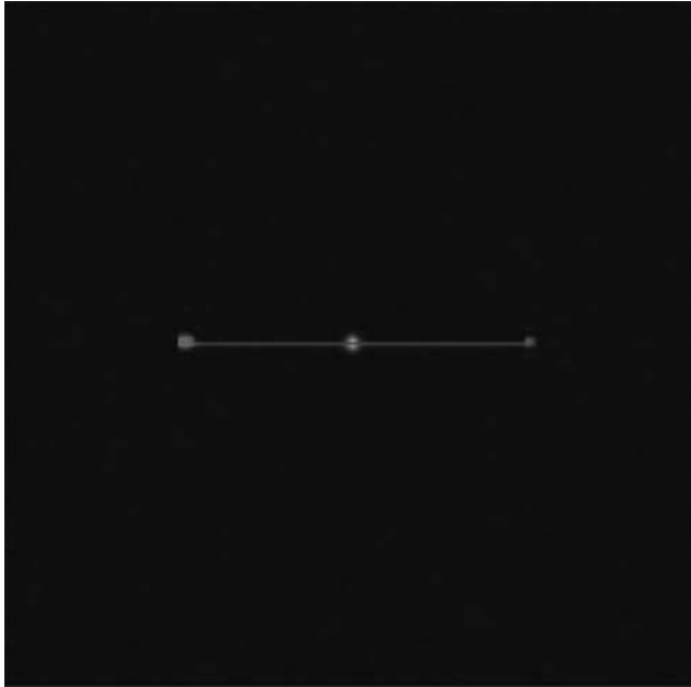
FIGURE 9.7 Autocorrelation of zero-mean random noise i(x, y) smoothed with a 9 \times 9 Gaussian filter.
